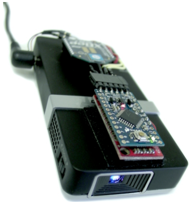
Figure 3. A 6DOF sensor is attached to the top of a handheld projector to sense user movement and gesture.
