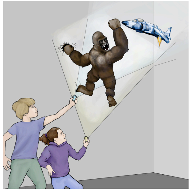
Figure 2: The SideBySide concept – a self-contained, full color, handheld projection device allowing multi-user interaction in almost any space.
