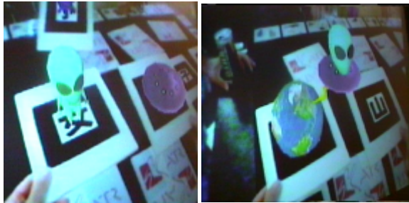
Figure 3: Spatial interaction in Shared Space: users trigger animation of virtual objects (in this case the alien and UFO) by bringing two cards together.
