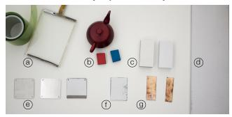
**Figure 7:** *REVEL Skins: a)* SiO<sub>2</sub> coated ITO panel and ITO rolls coated with vinyl; b) Anodized aluminum; c) Electro-coated aluminum; d) Drywall covered with copper emulsion and enamel paint; e) 3D printed resin, vacuum-plated and spray painted; f) Spray-painted nickel-plated ABS; c) vinyl and varnish coated copper plates.
