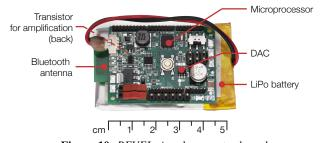
Figure 10: REVEL signal generator board.
