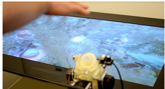
Figure 14: The user can feel textures of the virtual terrain.
