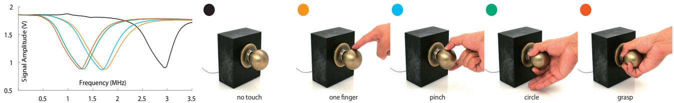
Figure 6: Capacitive profiles for making objects touch and grasp sensitive (doorknob example).
