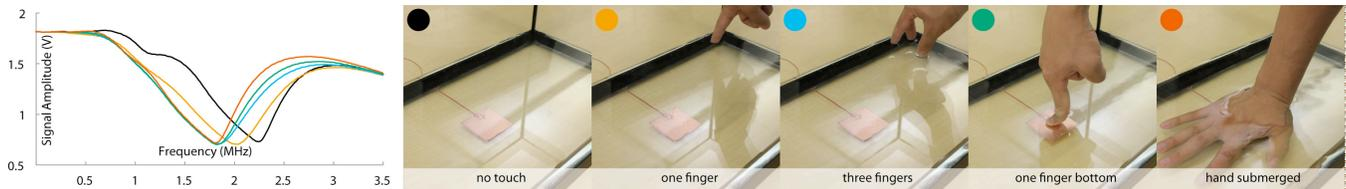
**Figure 10: Capacitive profiles for interacting with water.**
