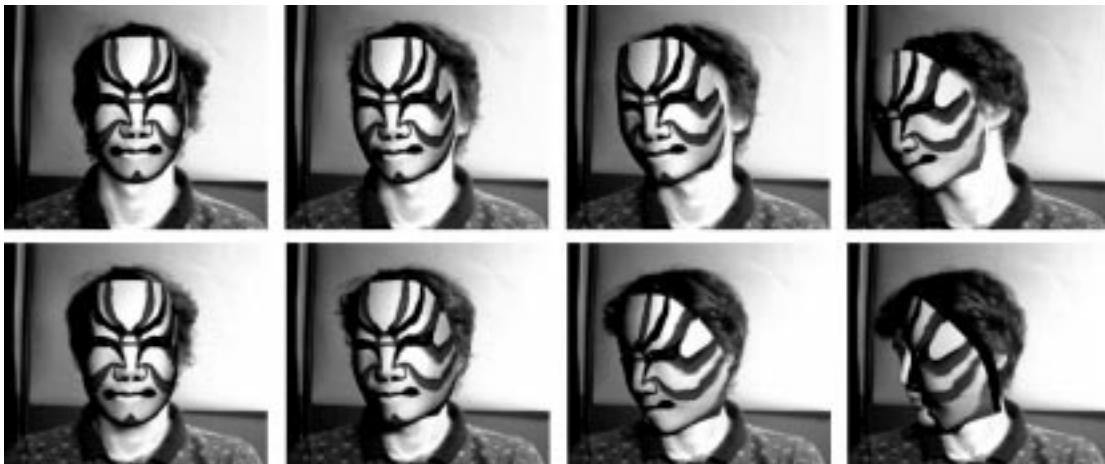
Figure 1: The rotation of a head mapped into mask rotations. Top row: the C-D gain was not used; the mask and face rotations are the same. Bottom row: the C-D gain was used, the mask rotates (non-linearly) further than the user's face.
