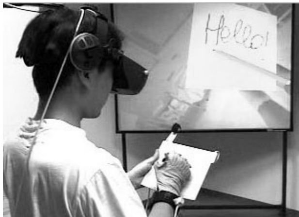
Figure 1. The physical setup of Virtual Notepad. The user is provided with a spatially-tracked tablet and pen for taking notes in the VRER.
